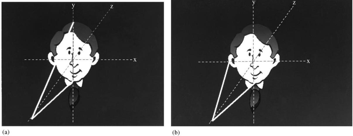
Fig. 2. Distance relationships from a camera viewpoint to two points on (a) the vertical axis (b) the horizontal axis.
