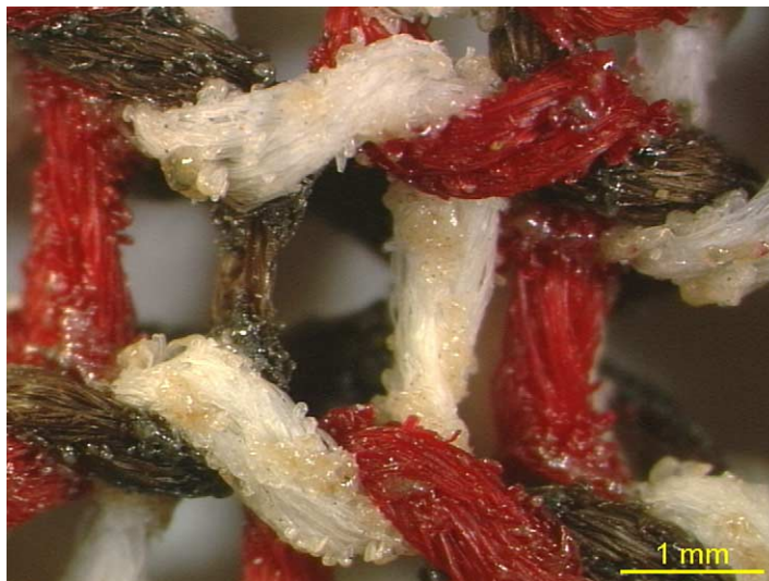
Fig. 5. Acrylic pullover subjected to vapour cloud explosion.
